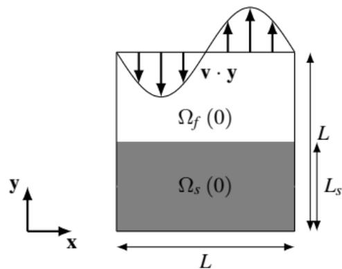
$$L = 1 \text{ m}, L_s = 0.5L, V_0 = 1 \text{ m} \cdot \text{s}^{-1}, \rho_f = \rho_s = 1 \text{ kg} \cdot \text{m}^{-3}, \nu_f = 0.001 \text{ Pa} \cdot \text{s}, \mu_s = 0.25 \text{ Pa}$$
